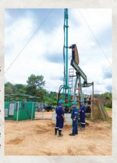
The long stroke, combined with the low pumping speed, will reduce friction and wear on the sucker rods against the tubing walls. This helps preserve the integrity of the system, extending its lifespan
