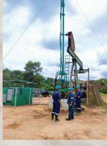
The long stroke, combined with the low pumping speed, will reduce friction and wear on the sucker rods against the tubing walls. This helps preserve the integrity of the system, extending its lifespan
